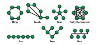
A **Network Topology** is the arrangement of the elements (links, nodes, etc.) of a communication network.
